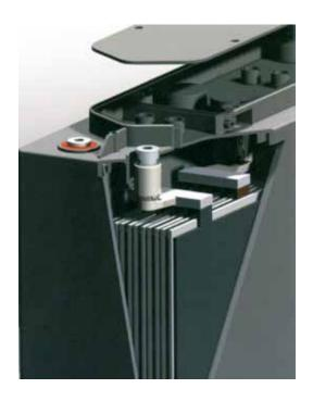
The front terminal AGM battery, designed for telecommunication applications with a floating life of up to 12 years, uses thickened 3D curved plates with special paste formula and latest AGM technology.
